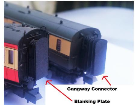
The blanking plate is needed to allow the gangway to smoothly rub against the coupled coach,
